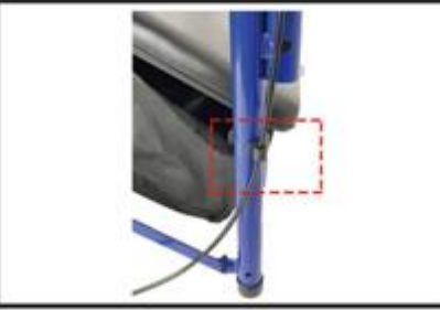
Using the cable clip to fix the cable properly
