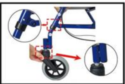
This part shall be facing outward,insert the front wheels to main frame
